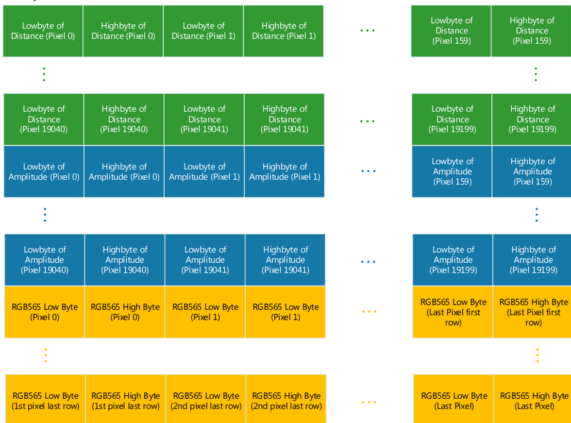
Figure 4-4: Data stream of Distance, Amplitude, RGB565 Color data
